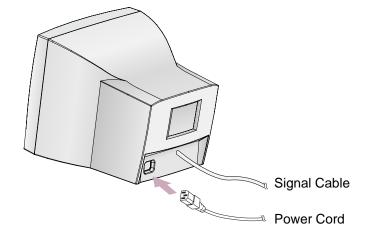
If your power cord is PC-to-Monitor type, plug the other end of the power cord into the AC receptacle in the computer.
